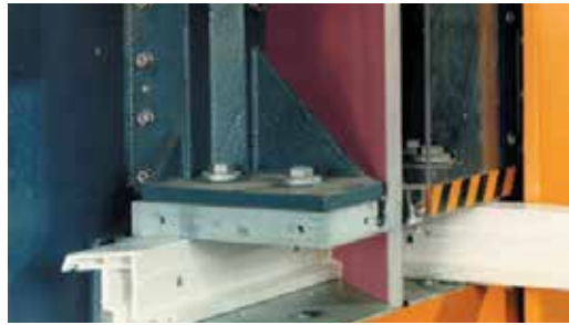
PVC extrusion welding, platen cover
